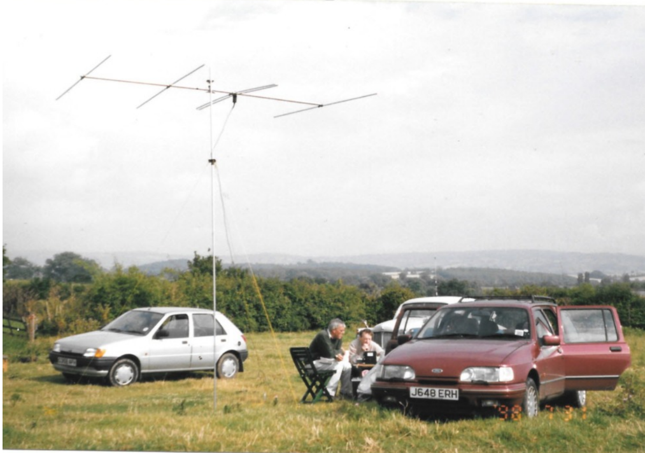
Brian G4CIB and Tony G4HBV operating on what appears to be 6 metres. The rig is an IC202S driving a 6m transverter into a 4 element yagi. The location is Gamage Court near Minsterworth, the QTH of Noel G4PHO (SK) , the year is 1998. (Photo 2E1GKY)
