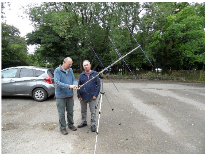
Here we see Dave G4BCA and Mike G6OTP with an Arrow 2m/70cm antenna with duplexer for satellite use. The antenna is feeding into a Kenwood TH-D72 handheld (Photo M0XAC)
