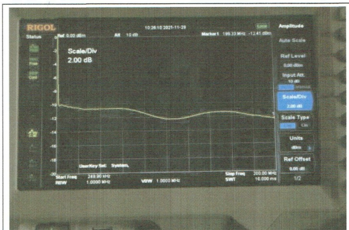
Figure 6: Response of attenuator from 250 kHz to 200 MHz with 10 dB attenuation added. Note that the vertical scale is now 2 dB per division, not 10 dB as in the previous figures.
