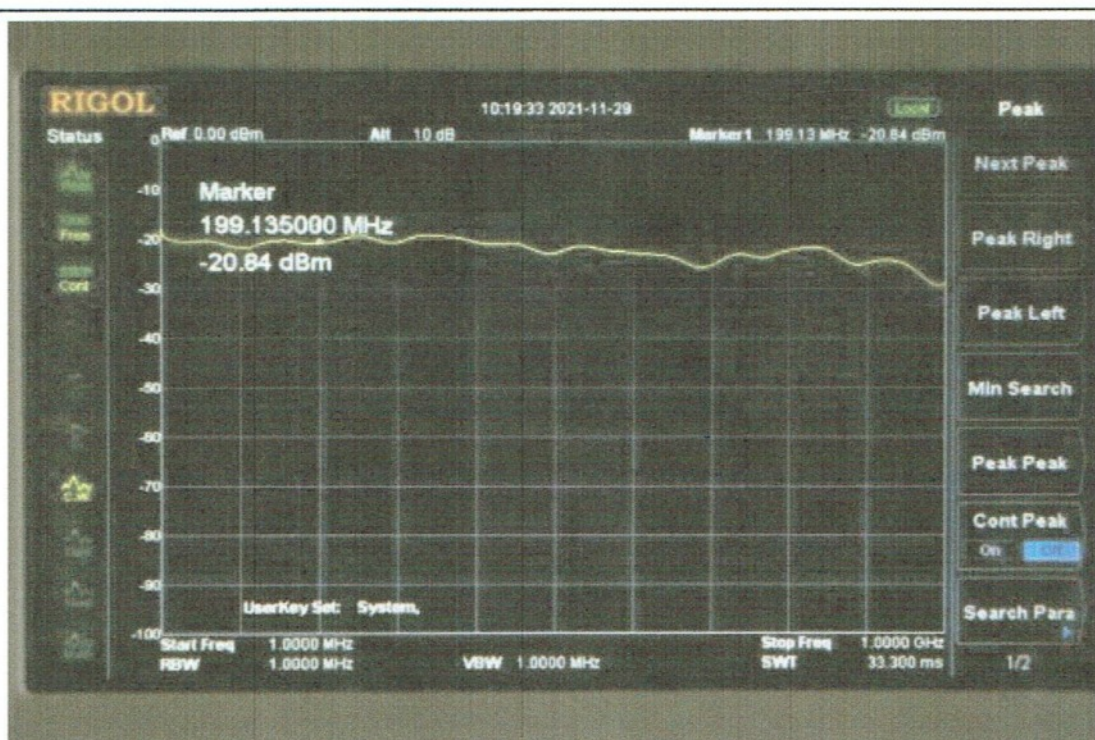
Figure 4: Response of attenuator from 1 MHz to 1 GHz with 20 dB attenuation added.
