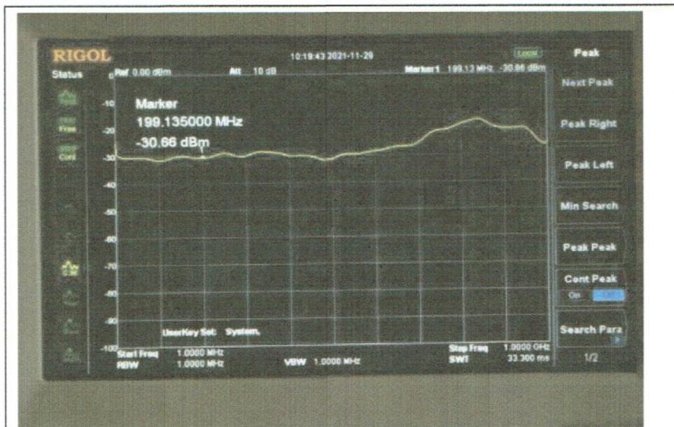
Figure 5: Response of attenuator from 1 MHz to 1 GHz with 30 dB attenuation added.
