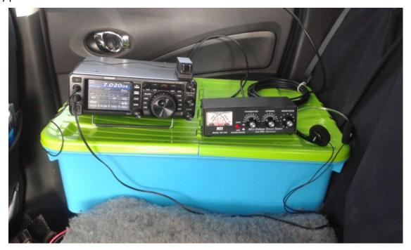
This photo above shows the 'station' on the back seat of the car comprising FT-991 and MFJ Travel Tuner (the latter only used for 40m). Note the Mini-Palm paddle which conveniently sits on top of the rig with a scratch-free magnetic base. The box contains everything needed for this type of operation (rig, magnetic mount, paddle, power cables, headphones, logbook and microphone for the rare occasions when I operate on SSB!).
