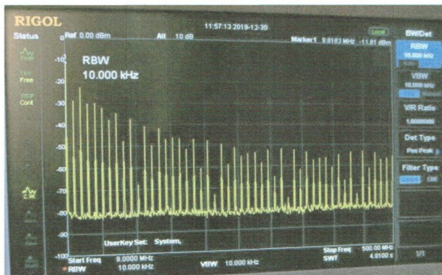
Figure 9: Output of TCXO, swept by spectrum analyser from 9 MHz to 500 MHz. The comb of harmonics is actually clearly visible in a wider sweep all the way out to 1 GHz. An external 20 dB attenuator was used for this measurement.
