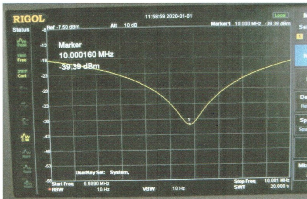
Figure 16: Bottom of crystal filter notch ( -39.4\ \text{dBm} ) swept over 2\ \text{kHz} range. Away from the notch, the level of attenuation (caused by two 4\ \text{dB} pi attenuator pads plus the transformer losses etc) was -9.5\ \text{dBm} so the attenuation at tuned frequency arising from the notch filter itself was 29.9\ \text{dB} .
