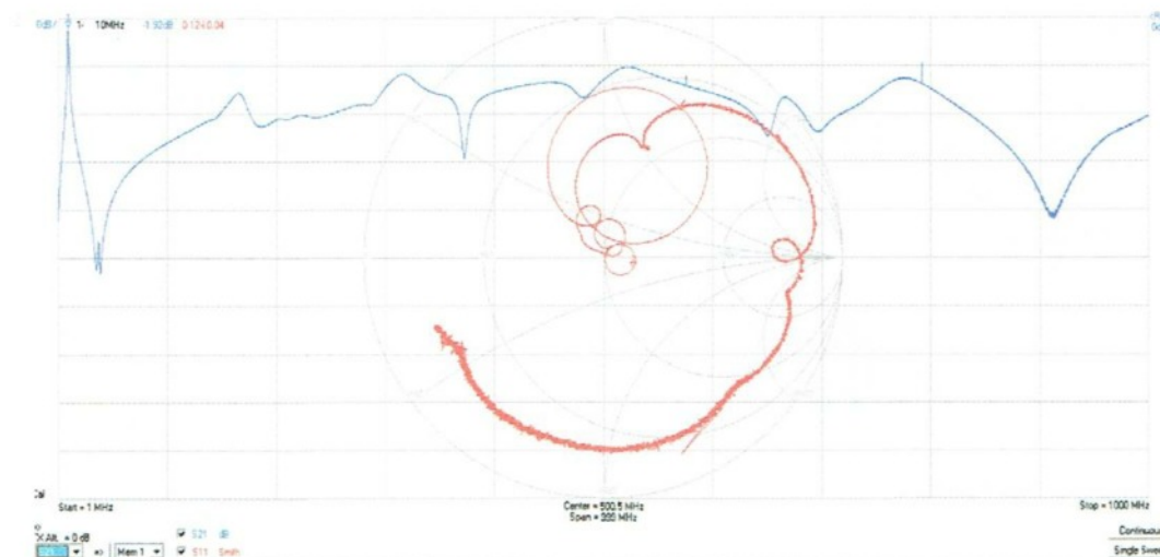
Figure 13: Diplexer test (blue trace showing insertion loss and red trace showing impedance on Smith Chart). Swept from 1MHz – 1 GHz.
