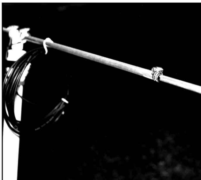
Figure 4—Complete the Simple Sixer by sliding in the narrower aluminum tubes and tightening the hose clamps.
