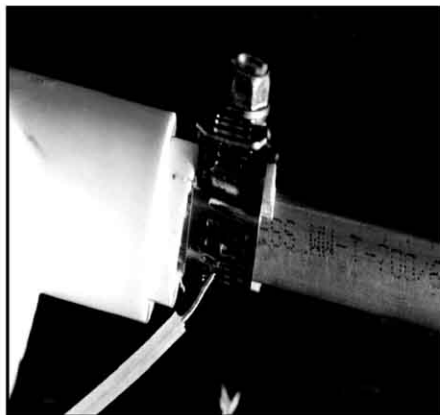
Figure 2—Use hose clamps to secure the aluminum tubing to the PVC T and to attach the coax conductors.
